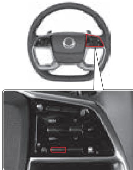
With Intelligent Speed Assistance set, pressing the right Intelligent Speed Assistance switch on the steering wheel will enable the function.
