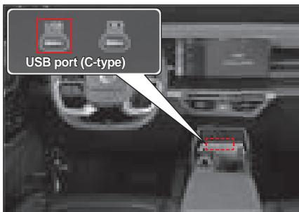
With the USB port, you can connect the external music / video playback devices such as USB storage and iPod to the vehicle.
