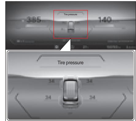
Select "Show Tire Pressure (TPMS)" from the instrument panel trip menu to view the pressure of all tires on the instrument panel.
