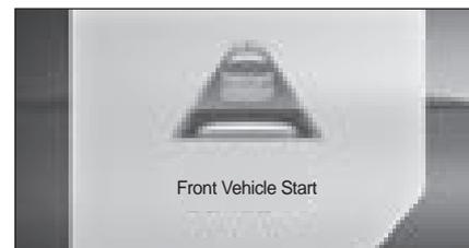
If the driver does not perform any operation (such as not starting the vehicle) about 1 second after the ahead vehicle departs, the message will be displayed on the LCD and alarm will sound.
