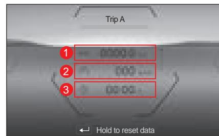
The distance that the vehicle traveled (km), average speed (km/h) and driving time (hh:mm) are displayed.
