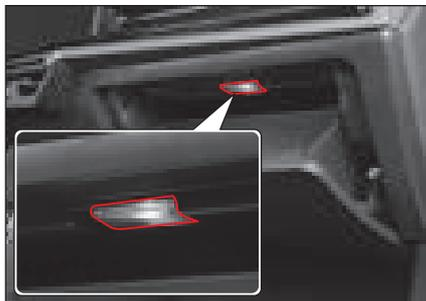
When you open the glove box, the lamp turns on, and when you close the glove box, the lamp turns off.
