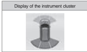
The distance from the obstacle is displayed on the instrument cluster along with the warning buzzer.
