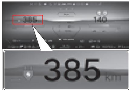
DTE shows the approximate distance your vehicle can travel before running out of power. The DTE value is calculated based on the current SoC of the HV battery, the driving mode (SPORT, ECO, ECO+), and the accumulated data on the driver's driving pattern.
