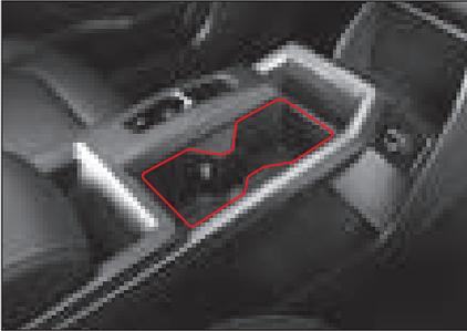
The cup holder is provided in front of the central console section.
