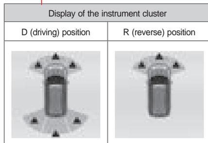
When the obstacle detection sensor is abnormal, “
