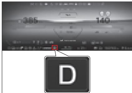
This indicator shows the current position of the electronic shift lever (P, R, N, D).
