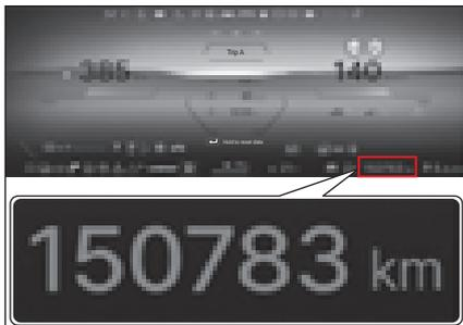
The total mileage of the vehicle is displayed in kilometers. The maximum mileage to be displayed is 999999 km.
