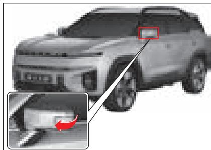
AUTO approach (outside rearview mirror unfolded) is activated when you are approaching within 1 m of the vehicle while carrying the smart key in theft deterrent mode.
