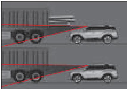
Caution should be taken that a tall vehicle or a vehicle with cargo sticking out the back of the vehicle may cause a dangerous situation.
