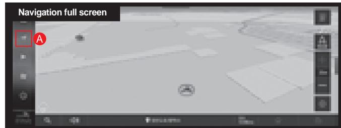
Lightly touch the navigation operation switch (A) to activate navigation.
