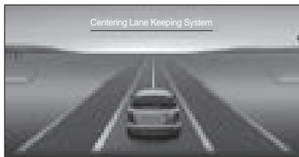
If only one lane is recognized at speeds above 40 km/h, only the recognized lane is colored green.
