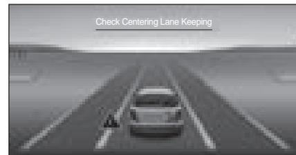
Displays if the Lane Keeping Assist (LKA) feature is undergoing a check.
