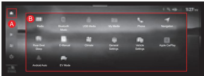
Lightly touch the Main Menu Controls switch (A) to display the switches (B) that allow you to set up your vehicle, which are detailed below.
