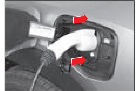
11 Align the charging connector to the charge port and insert completely.
