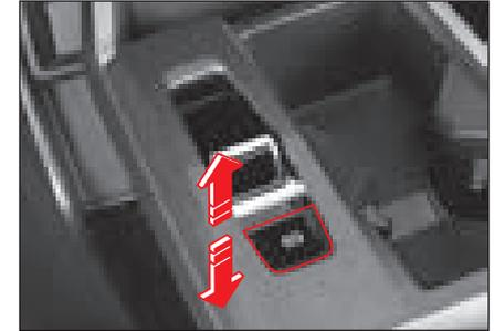
Operate the EPB (Electronic Parking Brake) switch and check the operating sound and operation status.
