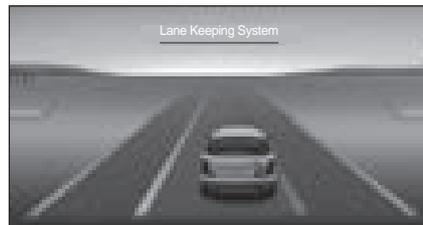
If your vehicle approach either side of the lane without turning on the corresponding turn signal lamp while the LKA is operating, the corresponding lane marker on the display will blink (green ↔ red).
