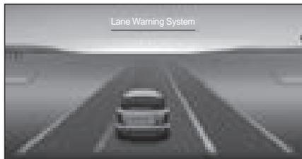
It is activated when the turn signal is not activated or the vehicle deviates from center of the lane.
