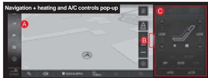
Touching the heater and air conditioner controls pop-up scroll (A) during navigation displays the heater and air conditioner controls panel (C).
