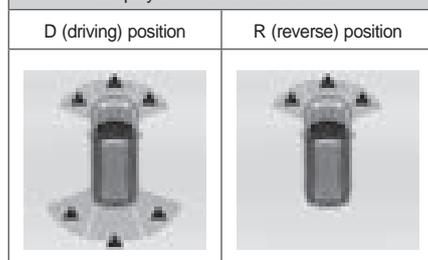
When the obstacle detection sensor is abnormal, “
