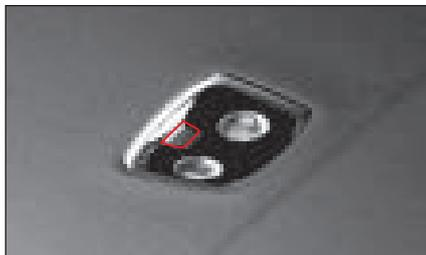
Pressing the center room lamp switch turns on the center room lamp. Pressing the switch again turns off the center room lamp. The center room lamp comes on when the door is opened regardless of the center room lamp switch operation if the door coupled switch is pressed in.
