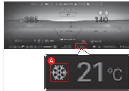
This Indicator displays the current ambient temperature.
