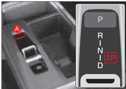
Select this position to park, start the vehicle, warm-up, and stop the vehicle for a long time.
