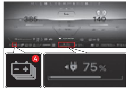
Indicates the state of charge of the high-voltage battery (drive battery).
