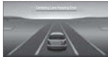
Displays if the Lane Keeping Assist (LKA) feature is unable to operate.
