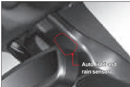
The auto light sensor is integrated with the rain sensor.
