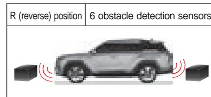
When the gear shift lever is placed in the R (reverse) position, 2 front obstacle detection sensors and 4 rear obstacle detection sensors are activated at the same time.
