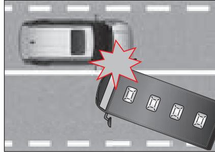
Since the impact of a collision in the diagonal direction is weaker than the impact of a collision in the front or side direction, the air bag may not inflate.
