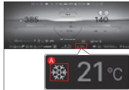
This Indicator displays the current ambient temperature.
