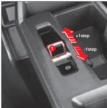
The electronic shift lever can be moved at + 1 step and - 1 step, after which it is always aligned to the central position.
