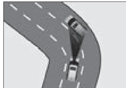
A vehicle on another lane may be detected, affecting the speed. Check the front road and driving conditions and adjust the vehicle speed directly by depressing the brake pedal if necessary.
