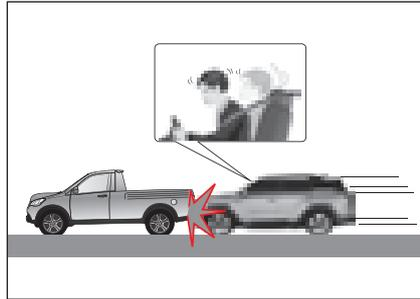
The air bag may not inflate in the event of a slight collision that the collision detection sensor cannot detect or the strength of collision is weak.
