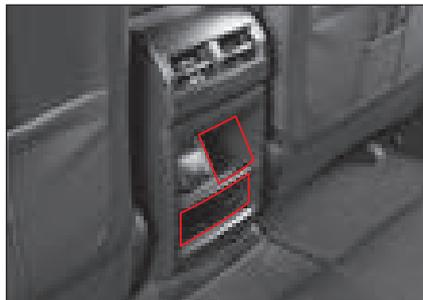
There is a pocket type storage box at the back side of the center console. This is suitable for storing small items.
