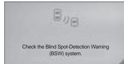
When the rear and side warning system is abnormal, a warning message is displayed on the display of the instrument cluster.
