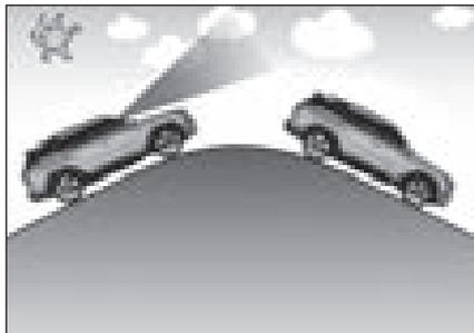
On a uphill road or a downhill road, a vehicle on the same lane cannot be detected and the AEBS performance is lowered so that unnecessary warning or braking is applied or the system may not operate.
