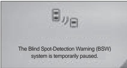
If the sensor cannot detect the rear and both side areas of the vehicle normally with the rear and side warning system activated, the message is displayed on the display of the instrument cluster.
