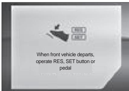
When the intelligent cruise control is operating, in congested areas, drive the vehicle while maintaining the distance to the front vehicle constant. Depress the accelerator pedal or push up the speed selector lever toward RES+ briefly or lower it toward SET- briefly to restart the vehicle 3 seconds after since the vehicle stops due to the front stationary vehicle.
