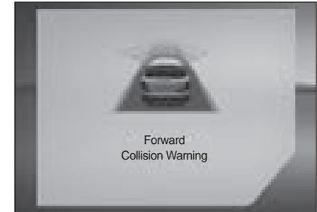
If the distance to the front vehicle is so close that a collision can occur or the front vehicle disappears from the front view due to lane change, etc. while the intelligent cruise control is activated, the message is displayed on the instrument cluster.
