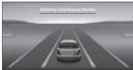
If your vehicle is traveling at a low speed (less than 40 km/h) or don't recognize both lanes, the lanes are shaded.
