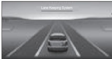
When both lane lines are detected while the vehicle is being driven at 40 km/h or more, both the lane markers on the display turns green.
