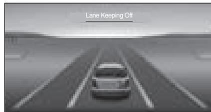
When the vehicle is driven at less than 40 kph (low speed conditions) or both lane lines are not detected, the lane marker is shaded.
