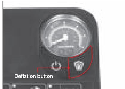
10 When the prescribed pressure is reached, press the power switch (1) of the service kit to turn it off.
