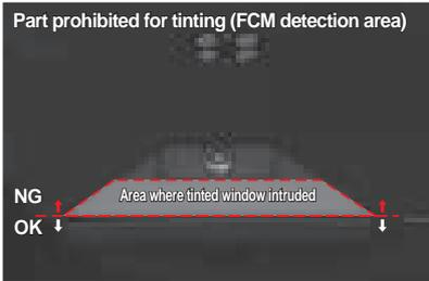
The diagram shows a top-down view of a vehicle's front camera field of view. A red trapezoidal area is outlined, representing the 'Area where tinted window intruded'. To the left of this area, there are two vertical arrows: a red one pointing up labeled 'NG' (Not Good) and a black one pointing down labeled 'OK'. The rest of the road surface is shown in grayscale.
