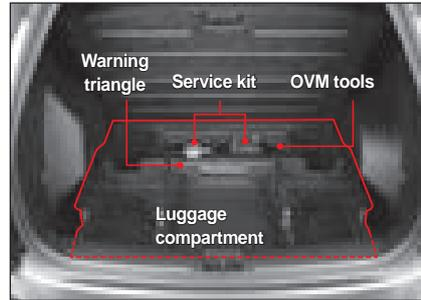
Below the luggage compartment board is a luggage compartment storage box for storing a warning triangle and OVM tools, including a service kit.
