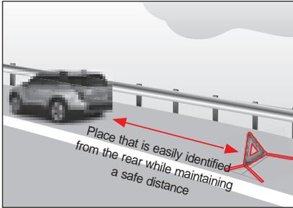
If the vehicle malfunctions and has stopped while driving, do not panic and take an action according to the following order.
