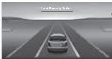
When only one lane line is detected while the vehicle is being driven at 40 km/h or more, the corresponding lane marker on the display turns green.
