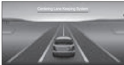
When both lanes are recognized at speeds above 40 km/h, both recognized lanes are colored green.
