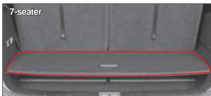
The size of the luggage board is different according to the space of the luggage compartment in the 5-seater vehicle and the 7-seater vehicle.
