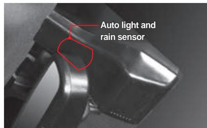
The rain sensor is integrated with the auto light sensor.
