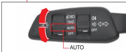
The auto light is the function that detects the amount of sunshine through the sensor and turns on or off the head light and the tail light automatically.
