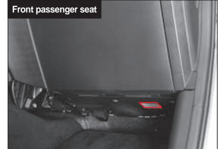
When you open the driver seat or front passenger seat door, the lamp turns on, and when you close the door, the lamp turns off.
