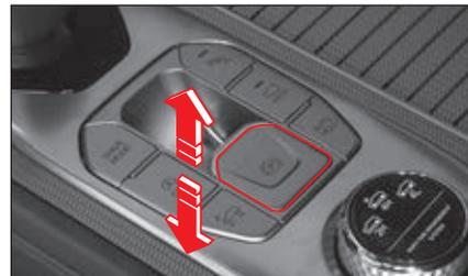
Operate the EPB (Electric Parking Brake) switch and check the operating sound and operation status.
