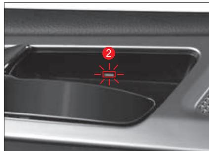
It turns on when the tail light is activated.
