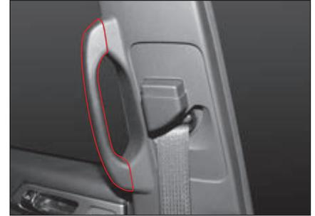
The grip handle is installed at the front of side of rear seats for convenience at the time of getting in and out of the vehicle.
