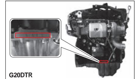
**Gasoline Engine:** The engine number is stamped on the bottom surface of the cylinder block behind the intake manifold.
