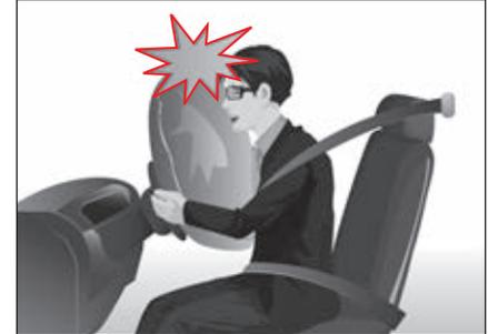
If the air bag control module detects the impact during an accident, it transmits the signal to deploy the air bag. This signal triggers the explosion of the powder, which is included in the air bag module, and the air bag deploys in a very short time to protect the occupants. When the air bag inflates, there will be heavy noise, glare and smoke. You could suffer secondary injuries caused by inflated air bag such as an abrasion, a bruise, a burn or injury by broken glasses.
