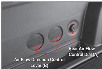
Air Flow Direction Control Lever (B)
