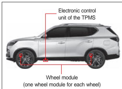
The electronic control unit of the TPMS receives various data including the tire pressure and temperature from the wheel module mounted on each wheel and displays such data on the instrument cluster.
