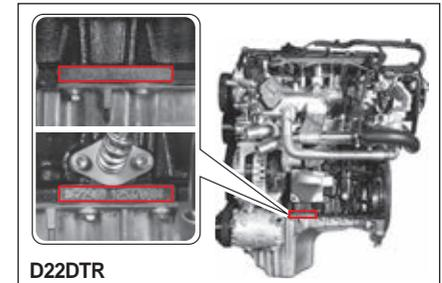
**Diesel Engine:** The engine number is stamped on the bottom surface of the cylinder block behind the exhaust manifold.
