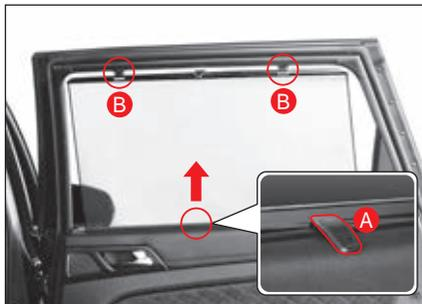
To block external light coming through the rear seat glass, operate the roller blind as follows:
