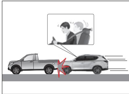
The air bag may not inflate in the event of a slight collision that the collision detection sensor cannot detect or the strength of collision is weak.
