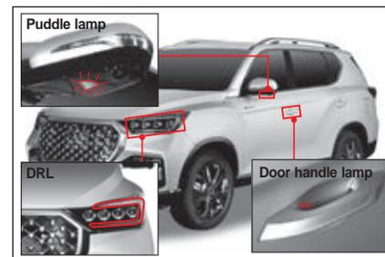
The welcome light is the function that operates the puddle lamp and the door handle lamp in order to increase safety and visibility at night.
