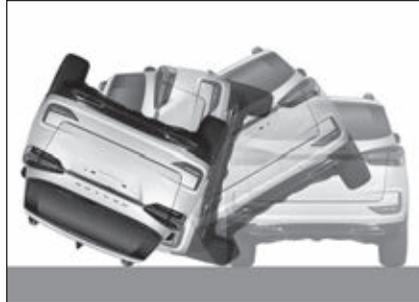
If the vehicle turns over or rolls over, the occupant cannot be protected fully by the air bag alone. In such case, the air bag may not inflate. However, the curtain air bag or the side air bag may inflate according to the degree of impact applied to the side when the vehicle turns over.
