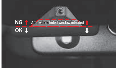
Part prohibited for tinting (FCM detection area)
